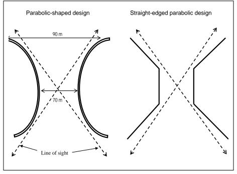
Parabolic-shaped overpass design and straight-edged design.
